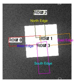
Illustration of the effect of sampling size along the edge of an MTF tool. Notice the color legend on left and right are different. On the right, ROI#1 is cropping the "East Edge", ROI#0 for "West Edge", ROI#2 for "North Edge" and ROI#3 for "South Edge", like you are reading a map normally. It is obvious that the longer the sample along the edge, the smoother the resultant MTF graphs.
