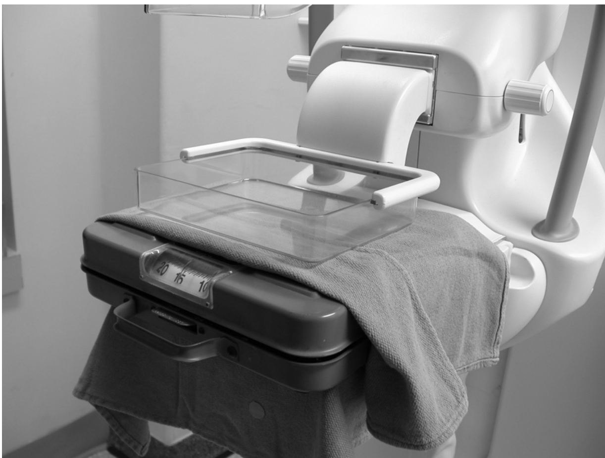
Figure 14: Positioning of bathroom scale to perform compression force measurement.
